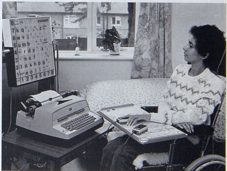
Sandra Bradbury using Possum GCTW12 scanning typewriter system (with TCPL1/2 input control)
